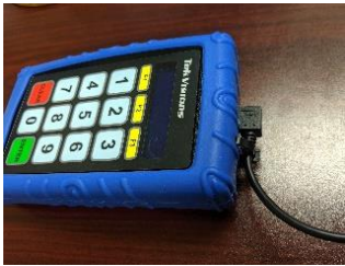
"Yank-Proof" Cable Management System (No Port Damage)
